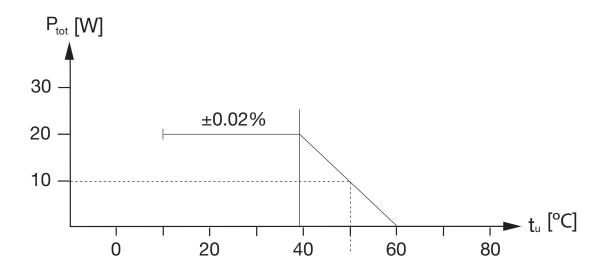
The load reduction curve can be used to find the maximum load that can be applied for different ambient temperatures for a given acceptable error arising from a load-induced rise. Example:  $t_u$  max. 50 °C, acceptable temperature-related  $\Delta R = 0.02$  %, gives a maximum permitted load of 10 W.
