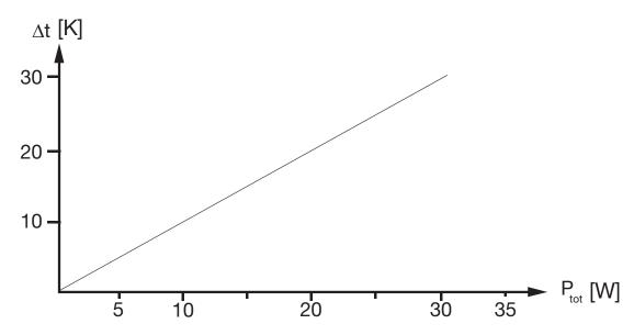
Heat-sink temperature = ambient temperature + temperature rise
