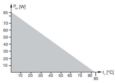
At an ambient temperature of 85 °C, no more than "0 W" is allowed to be input (in theory).
