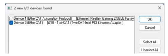
At this point you are to perform a device search by confirming the Scan for boxes request or later by right-clicking on the found EtherCAT device and selecting Scan in the context menu as shown below:
