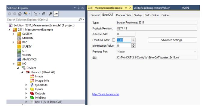
Build the project via Build → Build Solution, click on the Login = symbol and set a break point (F9) in the first code line:
