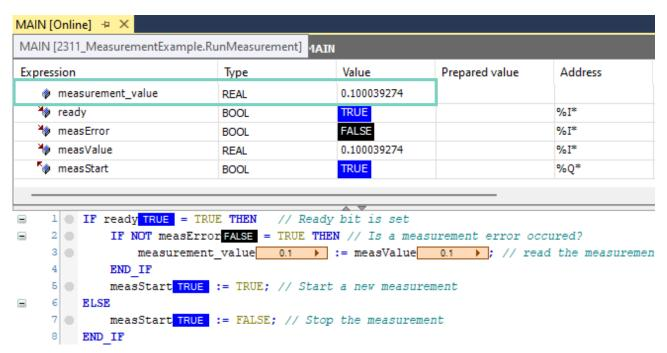
Note: If measurement does not start: please make sure that Control via EtherCAT is selected in device
