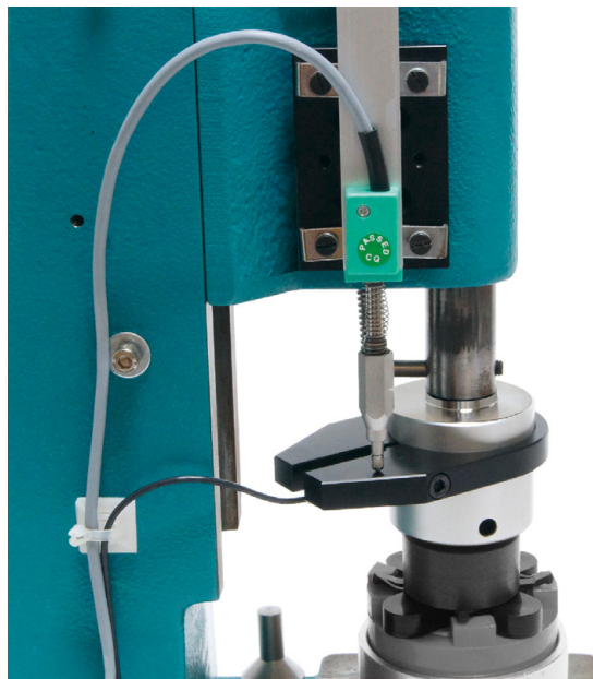
Displacement measurement system (DMS) in the lower position
