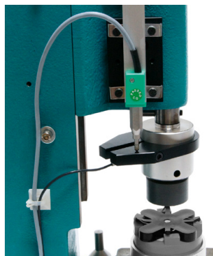
Displacement measurement system (DMS) in the upper position
