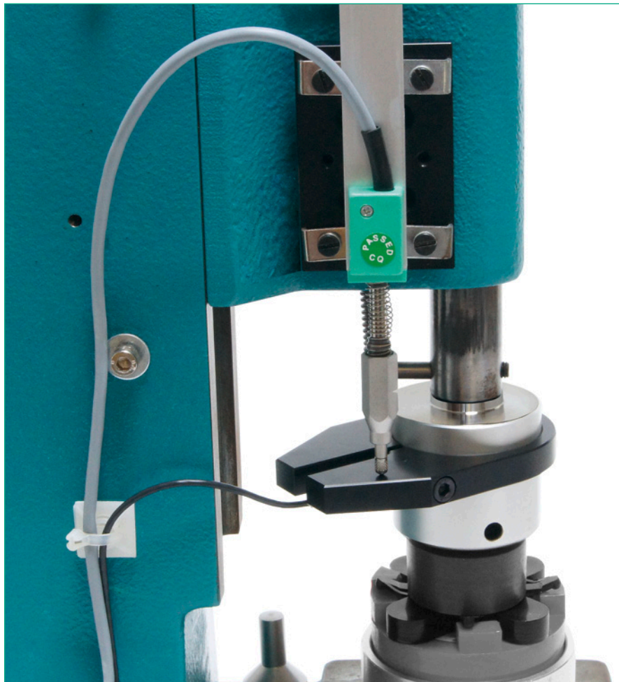
Figure 1.6: Displacement measuring system in the lowered position
