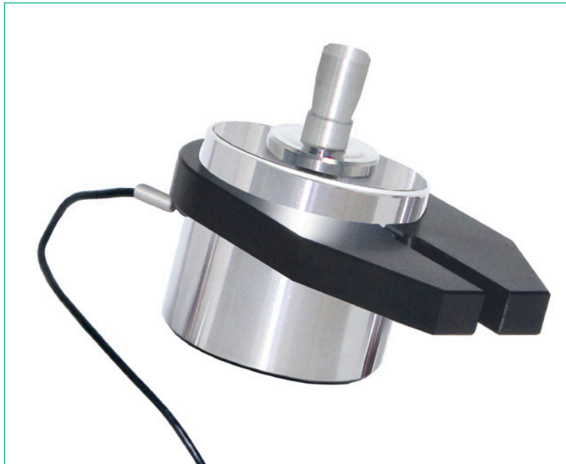
Figure 1.1: Fitting the carrier on the load cell
