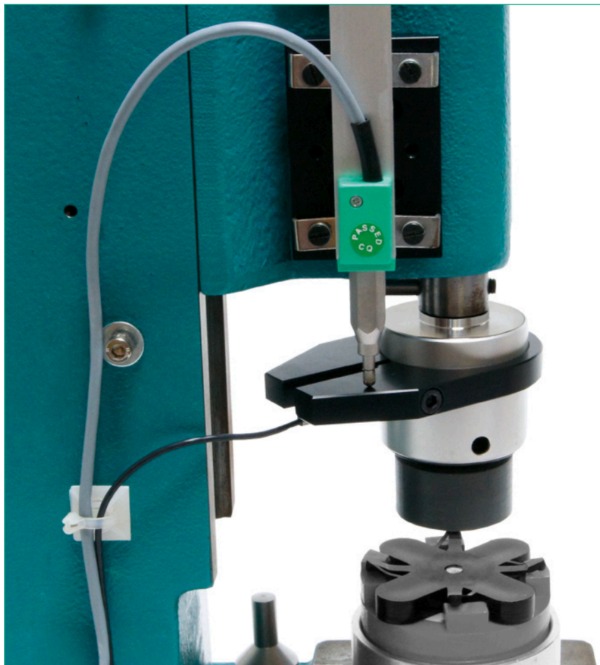
Figure 1.5: Displacement measuring system in the raised position
