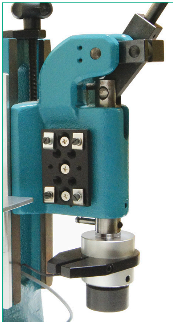
Figure 1.4: Displacement measuring system on the press
