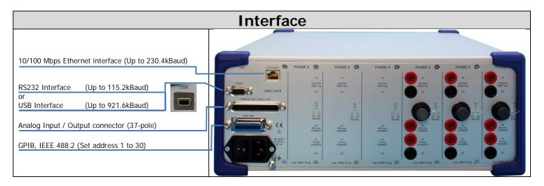
Servicing: Replacement amplifier boards from the factory are calibrated (no re-calibration is required). All other boards can simply be exchanged. Calibration: Use computer software, follow calibration instructions. Apply 60Hz, 1.5mA - 20A, and 0.3V - 1000V. Calibration cycle 2 years.
